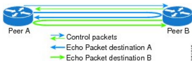
Figure 18: BFD Asynchronous Mode With Echo Packets
