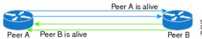
Figure 17: BFD Asynchronous Mode Without Echo Packets
