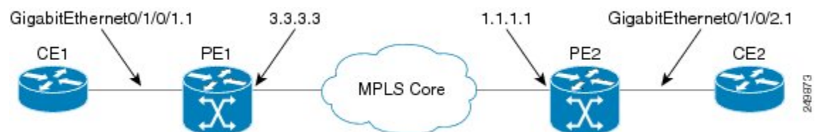
Figure 37: VPLS with BGP autodiscovery and BGP signaling
