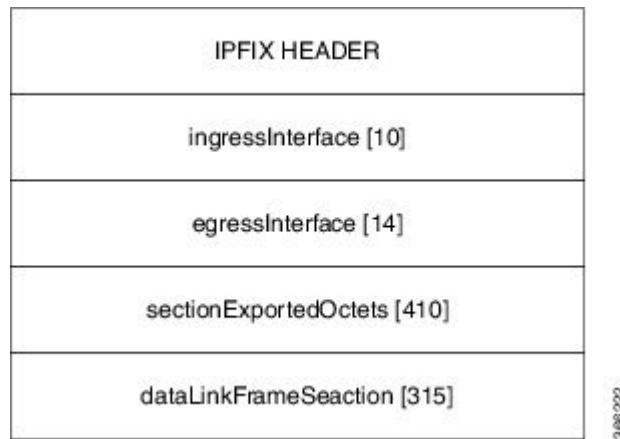
Figure 4: IPFIX 315 Export Packet Format
