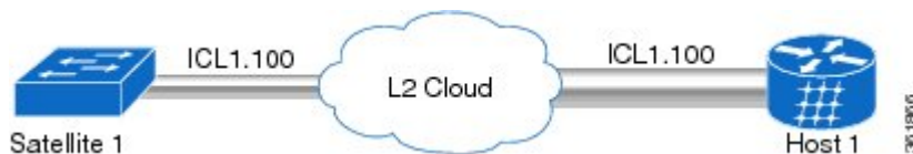
Figure 6: Layer 2 Fabric Single Home (SH) with Single Physical ICL on Host and Satellite
