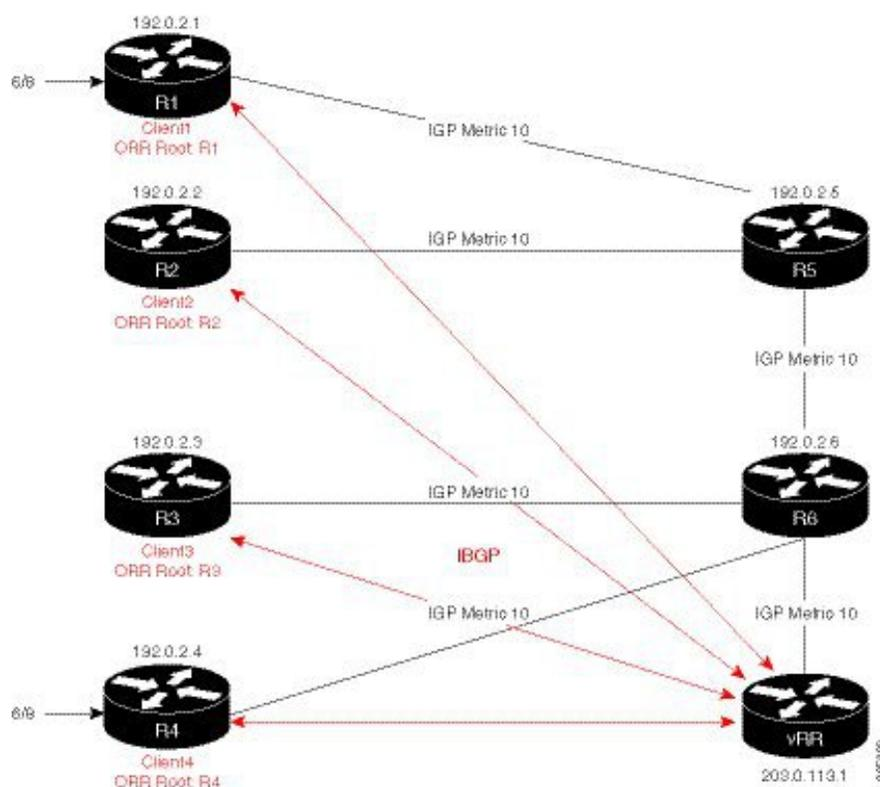
Without BGP ORR configured in the network, the vRR selects R4 as the closest exit point for RR clients R2, R3, R5, and R6, and reflects the 6/8 prefix learned from R4 to these RR clients R2, R3, R5, and R6. From the topology, it is evident that for R2 the best path is R1 and not R4. This is because the vRR calculates best path from the RR's point of view.
