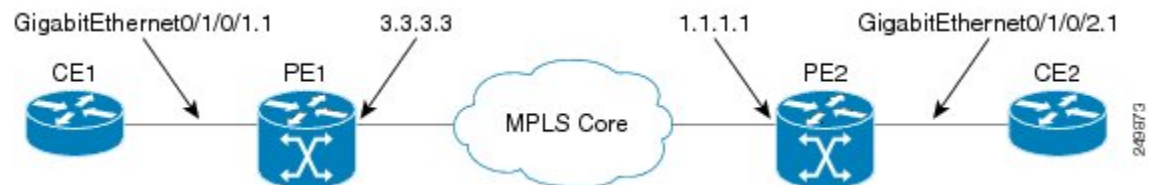
Figure 37: VPLS with BGP autodiscovery and BGP signaling
