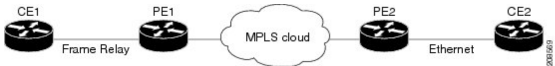
Figure 9: IP Interworking Over MPLS
