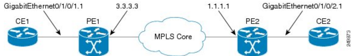
Figure 38: VPLS with BGP autodiscovery and BGP signaling
