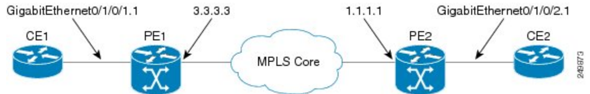
Figure 38: VPLS with BGP autodiscovery and BGP signaling
