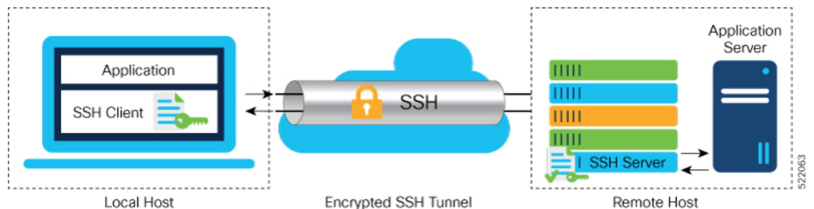
Figure 15: SSH Port Forwarding
