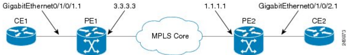
Figure 38: VPLS with BGP autodiscovery and BGP signaling
