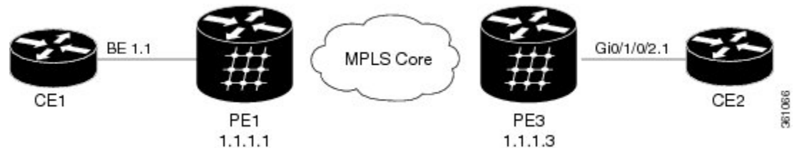
Figure 53: PBB-EVPN on Single Homed Device/Single Homed Network
