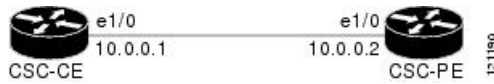
Figure 39: Configuration for Peering with Directly Connected Interfaces Between CSC-PE and CSC-CE Routers
