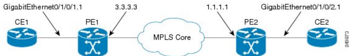
Figure 21: VPLS with BGP autodiscovery and BGP signaling
