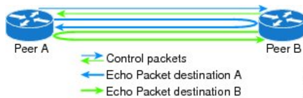
Figure 15: BFD Asynchronous Mode With Echo Packets
