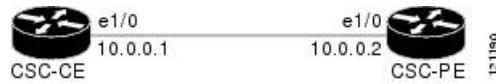
Figure 40: Configuration for Peering with Directly Connected Interfaces Between CSC-PE and CSC-CE Routers
