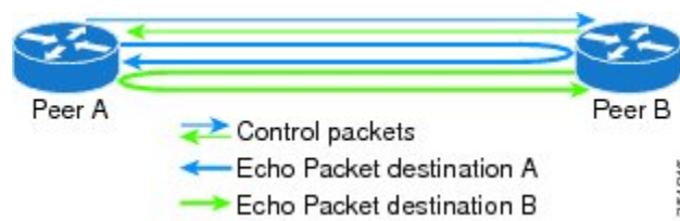
Figure 14: BFD Asynchronous Mode With Echo Packets
