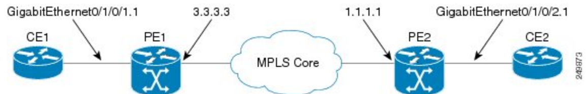
Figure 21: VPLS with BGP autodiscovery and BGP signaling
