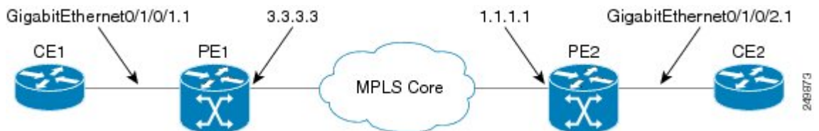
Figure 21: VPLS with BGP autodiscovery and BGP signaling
