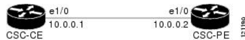
Figure 39: Configuration for Peering with Directly Connected Interfaces Between CSC-PE and CSC-CE Routers
