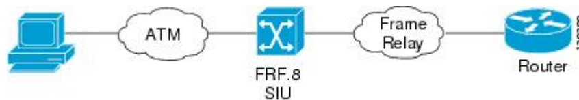
Figure 11: Frame Relay-to-ATM Interworking
