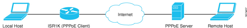
Figure 30: Sample Topology of a PPPoE Client and Server over a VLAN Interface
