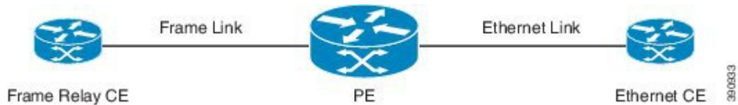
Figure 47: Frame Relay-Ethernet Local Switching Topology
