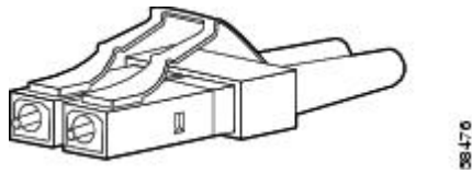
Figure 2: Fiber-Optic SFP Module LC Connector
