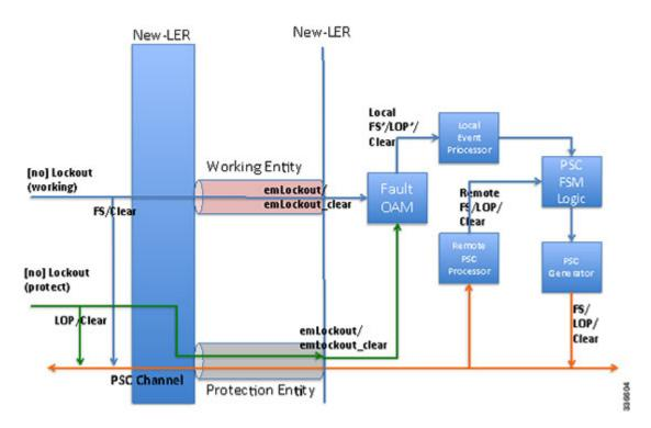
When a lockout (working) command is issued, the new-LER implementation sends an emLockout command on the working LSP and PSC(FS) on the protected LSP. The remote peer receives two commands in either order. A priority scheme for local events is modified slightly beyond what is defined in order to drive the PSC FSM to a consistent state despite the order in which the two messages are received.
