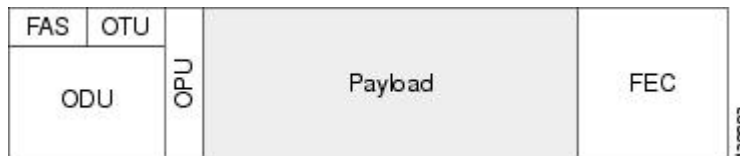
Figure 1: OTN Optical Channel Structure
