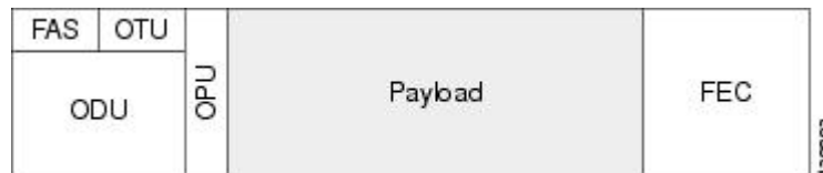
Figure 2: OTN Optical Channel Structure
