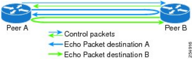
Figure 9: BFD Asynchronous Mode With Echo Packets
