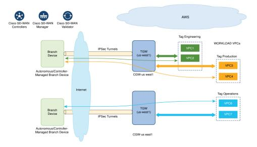
The SD-Routing branch device can have only the default VRF. You can use this default VRF to mapping through the SD-Routing Cloud OnRamp branch connect. You cannot use any other VPN/VRF for mapping. Along with SD-Routing soluction, you can have multiple VPN mapping for SD-WAN solution. Both the Cisco SD-WAN and Cisco SD-Routing connection can co-exist.
