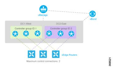
You configure the three vSmart controllers in DC1-West with controller group identifier 1:
