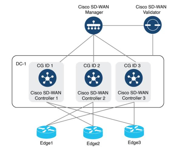
To display the control connections with the Cisco SD-WAN Controllers, use the **show control connections** command. The last column on the output, **Controller Group ID**, lists the Cisco SD-WAN Controller group that a router is in.
