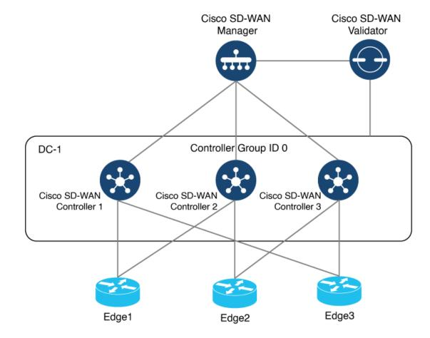
In the topology that is shown in the figure above, there are three Cisco SD-WAN Controllers in Data Center DC-1, all of which belong to default controller group 0. A Cisco vEdge device selects two Cisco SD-WAN Controllers, which are identified as its assigned Cisco SD-WAN Controllers. Each tunnel interface of the Cisco vEdge device connects to these assigned Cisco SD-WAN Controllers. When a tunnel interface connects to its assigned Cisco SD-WAN Controllers is assigned Cisco SD-WAN Controllers.
