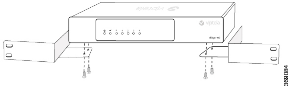
Figure 7: Attaching the Mounting Ears to the vEdge 100 Router Chassis
