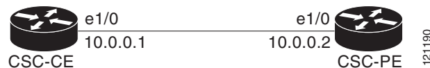
Figure 37 Configuration for Peering with Directly Connected Interfaces Between CSC-PE and CSC-CE Routers
