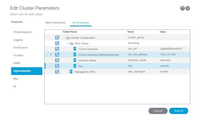
Step 3 The management IP address of the LDev becomes the virtual IP address of the ASA cluster. The primary control unit gets a separate IP address as its local IP address once the cluster is formed. Change the IP address of the CDev representing the primary control unit to the new local IP address. Otherwise, the APIC is not able to monitor the health of the primary control unit if there is a change of primary control unit such as during a failover.
