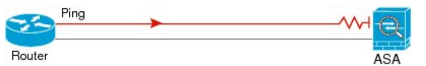
Figure 75: Ping Failure Because the ASA Has No Return Route
