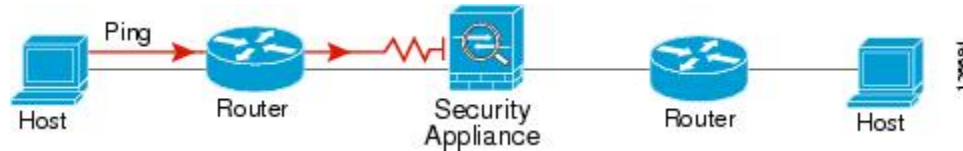
Figure 76: Ping Failure Because the ASA is Not Translating Addresses
