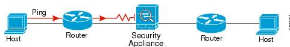
Figure 73: Ping Failure Because the ASA is Not Translating Addresses
