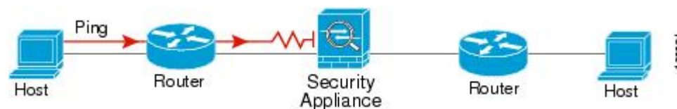
Figure 79: Ping Failure Because the ASA is Not Translating Addresses
