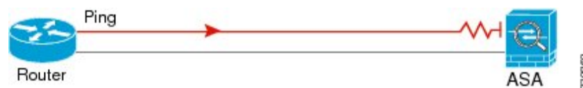
Figure 93: Ping Failure Because the ASA Has No Return Route
