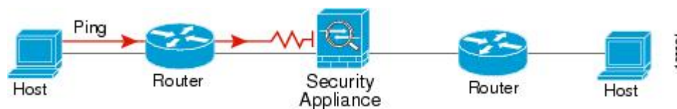
Figure 82: Ping Failure Because the ASA is Not Translating Addresses
