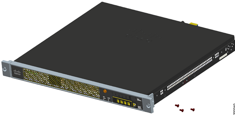
Figure 6 Install Die-Cast Brackets with Three Screws
