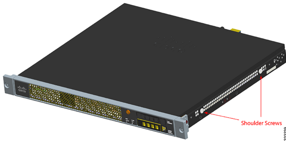
Figure 7 Install Two Shoulder Screws on Either Side of the Chassis
