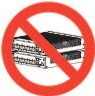
Figure 1: Do Not Stack the ASA Chassis
