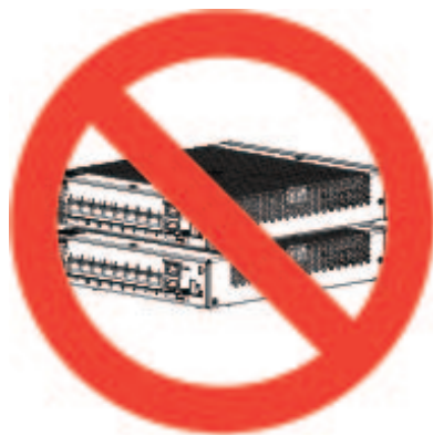
Figure 23: Do Not Stack the Chassis
