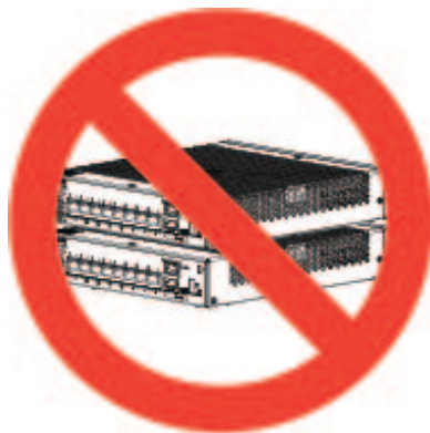
Figure 24: Do Not Stack the Chassis
