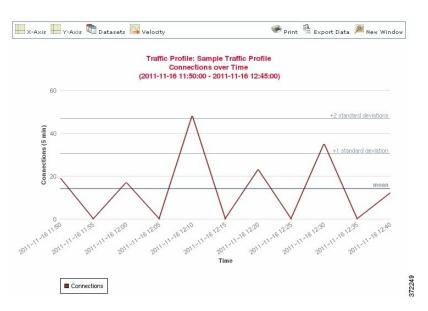
You can also set up inactive periods in traffic profile. Traffic profiles collect data during inactive periods, but do not use that data when calculating profile statistics. Traffic profile graphs plotted over time show inactive periods as a shaded region.
