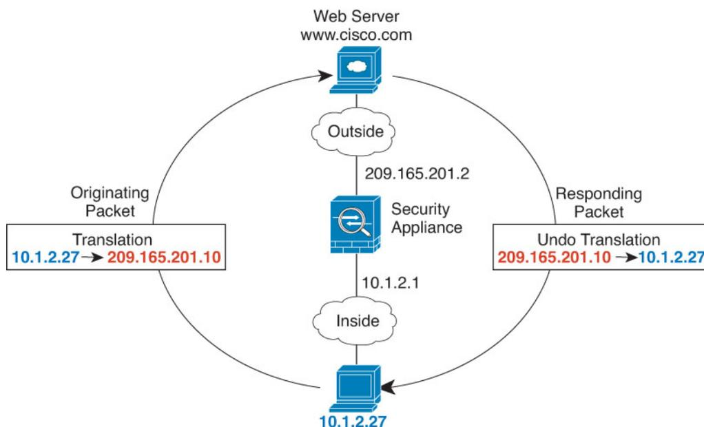
1. When the inside host at 10.1.2.27 sends a packet to a web server, the real source address of the packet, 10.1.2.27, is translated to a mapped address, 209.165.201.10.
