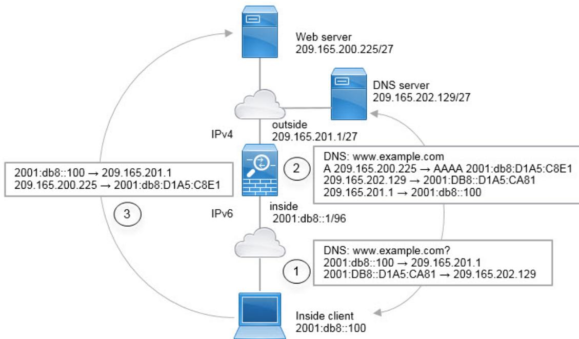
In this example, you translate the inside IPv6 network to IPv4 using dynamic interface PAT with the IP address of the outside interface. Outside IPv4 traffic is statically translated to addresses on the 2001:db8::/96 network, allowing transmission on the inside network. You enable DNS rewrite on the NAT46 rule, so that replies from the external DNS server can be converted from A (IPv4) to AAAA (IPv6) records, and the addresses converted from IPv4 to IPv6.
