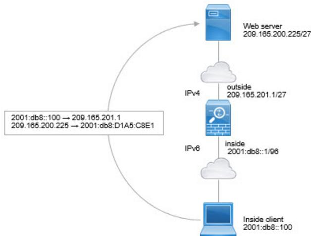
In this example, you translate the inside IPv6 network to IPv4 using dynamic interface PAT with the IP address of the outside interface. Outside IPv4 traffic is statically translated to addresses on the 2001:db8::/96 network, allowing transmission on the inside network.
