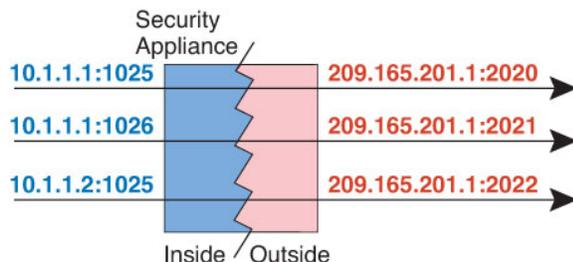
For the duration of the translation, a remote host on the destination network can initiate a connection to the translated host if an access rule allows it. Because the port address (both real and mapped) is unpredictable, a connection to the host is unlikely. Nevertheless, in this case you can rely on the security of the access rule.
