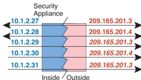
Instead of using a static rule this way, we suggest that you create a one-to-one rule for the traffic that needs bidirectional initiation, and then create a dynamic rule for the rest of your addresses.
