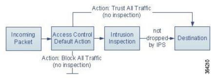
Note that only ASA FirePOWER modules deployed inline can affect the flow of traffic. Applying an access control policy configured to block or alter traffic to passively deployed devices can have unexpected results.
