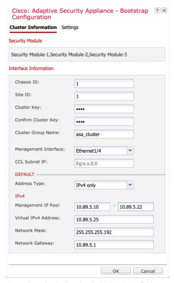
a) For inter-chassis clustering, in the **Chassis ID** field, enter a chassis ID. Each chassis in the cluster must use a unique ID.
