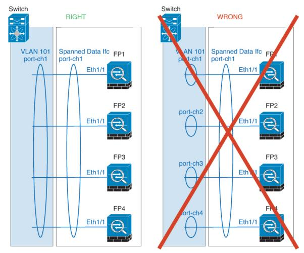
• Device-local EtherChannels—For cluster unit *Device-local* EtherChannels including any EtherChannels configured for the cluster control link, be sure to configure discrete EtherChannels on the switch; do not combine multiple cluster unit EtherChannels into one EtherChannel on the switch.
