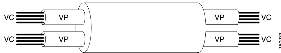
Figure 62-2 ATM Virtual Path and Virtual Channel Connections
