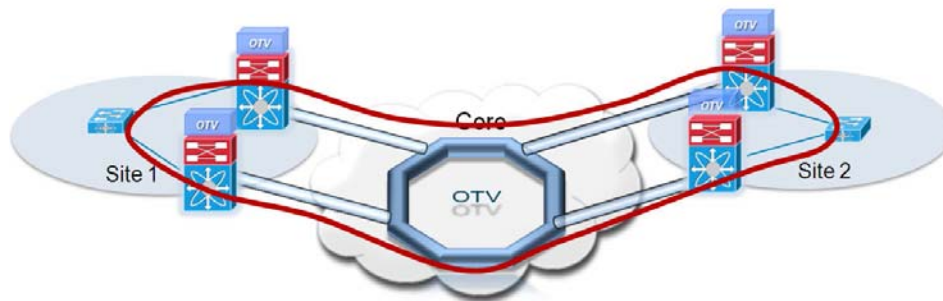
Figure 1-22 Creation of an End-to-End STP Loop
