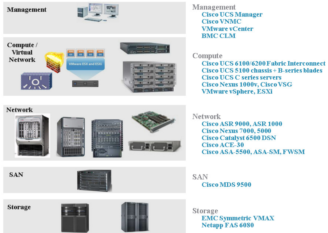
Figure 3-1 VMDC Infrastructure Components
