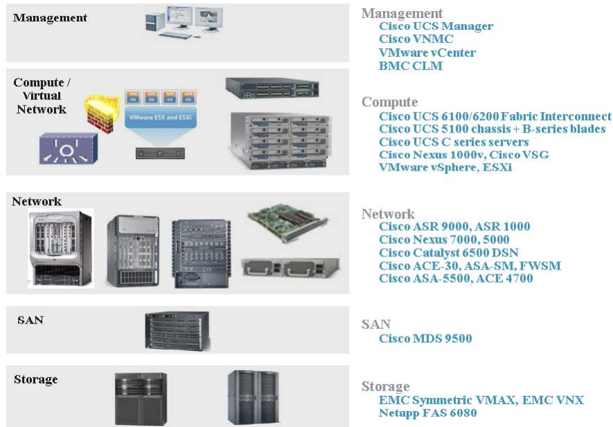
Figure 2-1 VMDC Infrastructure Components
