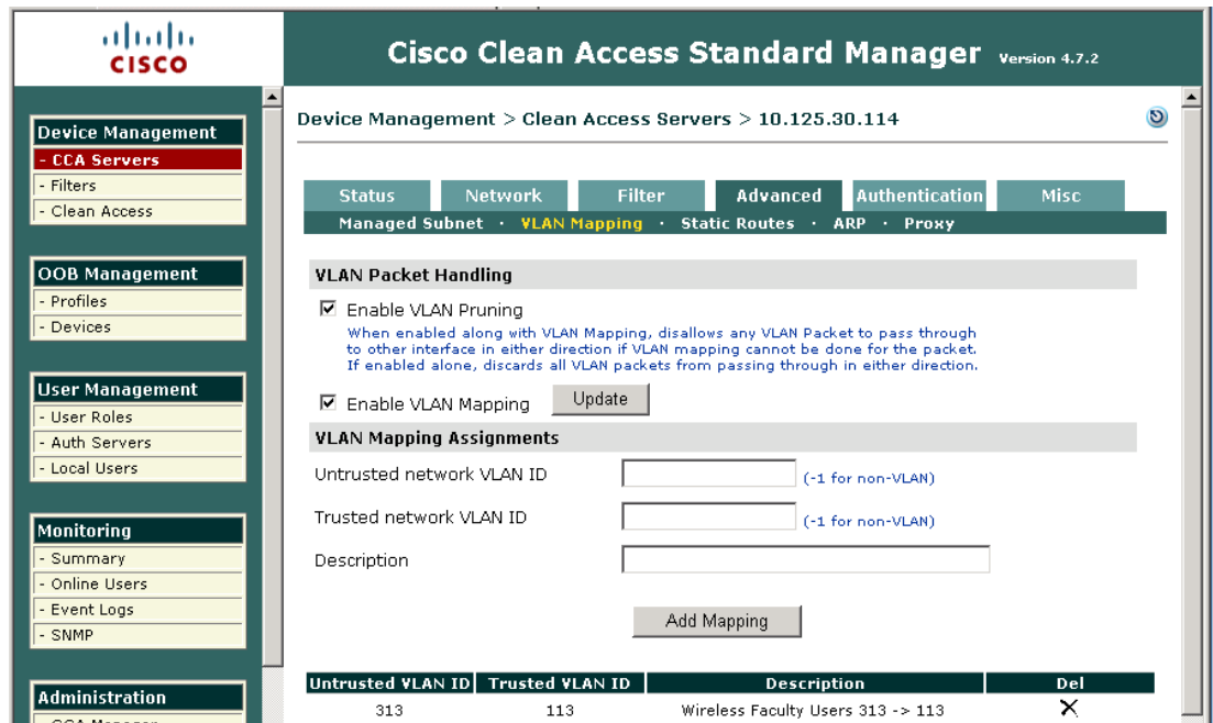
Figure 6-68 Creating VLAN Mappings
