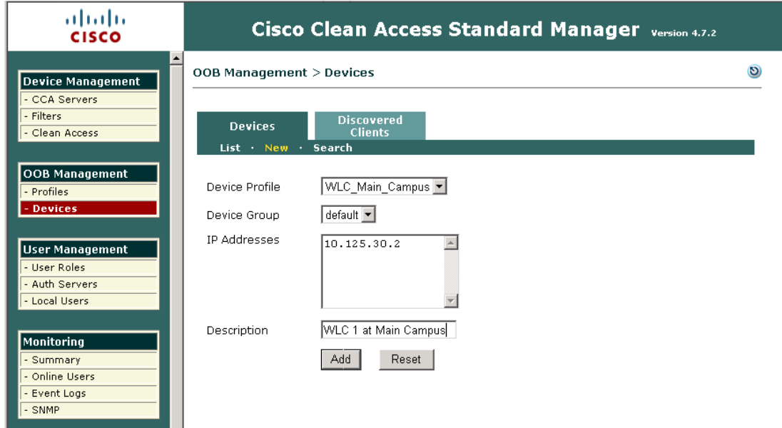
Figure 6-61 Adding WLC in Profile
