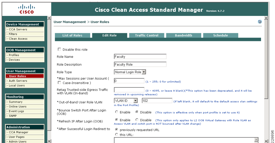
Figure 6-55 Creating Faculty Role and Mapping it to VLAN 102
