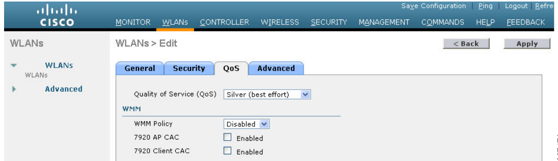
Figure 5-19 Secured Staff WLAN QoS
